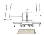
To enable the tank to be unloaded, a distance of 6m in diameter around the truck will be required. This will also allow enough distance for the crane's outriggers (legs).
