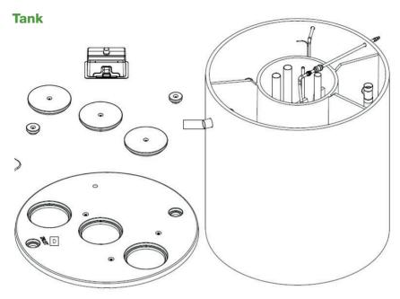
Precast tank external dimensions  $2.4m \text{ dia} \times 2.4m \text{ high} + \text{tank lid } .75m = 3.15m \text{ total height}$
